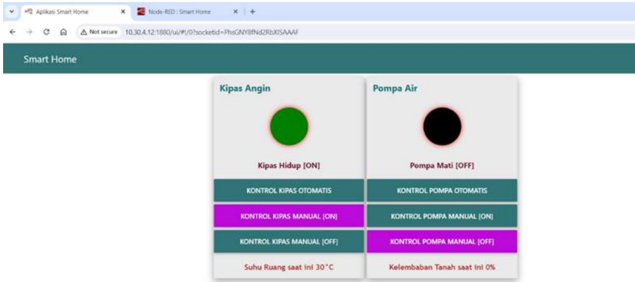
Fig 3. Node-RED Dashboard Display for Monitoring and Controlling the Fan.
