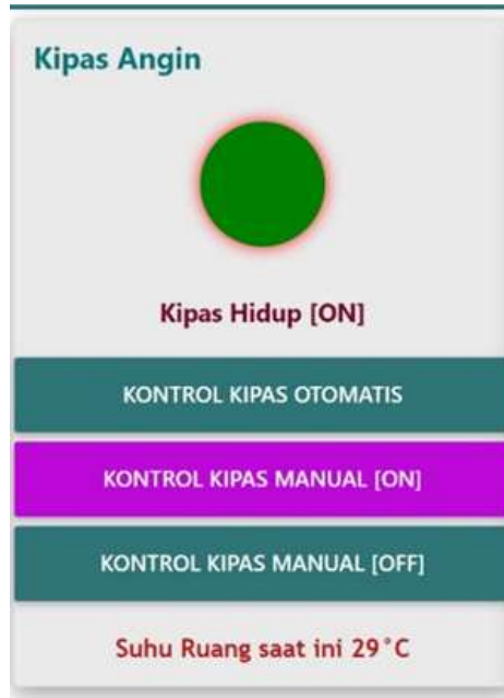
Fig 5. Node-Red Dashboard Output Display in Manual Testing ON
