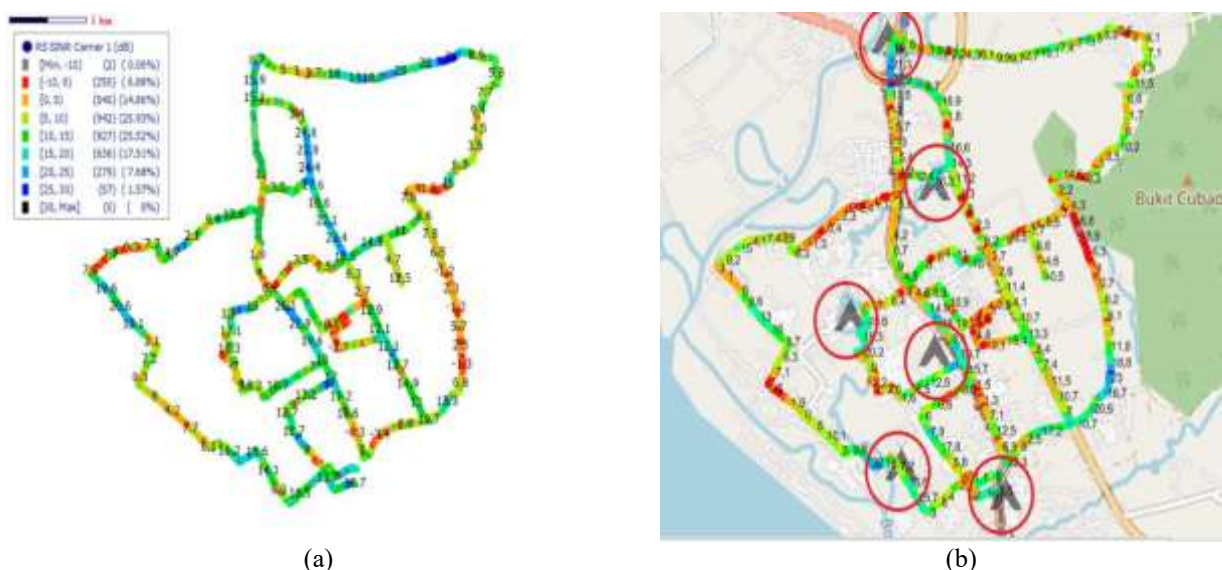
Fig. 10 (a) Drive test results on SINR Operator Telkomsel, (b) Drive test results on SINR Operator Tri
